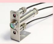
DLSBFS Dual laser sighting bracket, fixed DLSBAS Dual laser sighting bracket, adjustable DLSBCE Extended cable - 1 m
