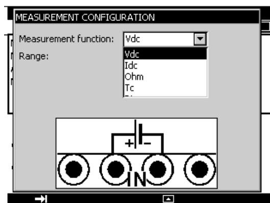
Connections in the measurement mode are made to the four "IN" terminals on the left half of the unit:
