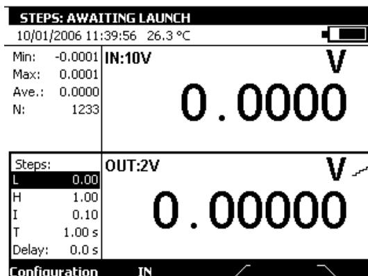
The function key launches a cycle of increasing increments and the function key launches a cycle of decreasing increments.
