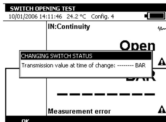
To accept (acknowledge) the measurement, press the function button, **F1** (OK).
