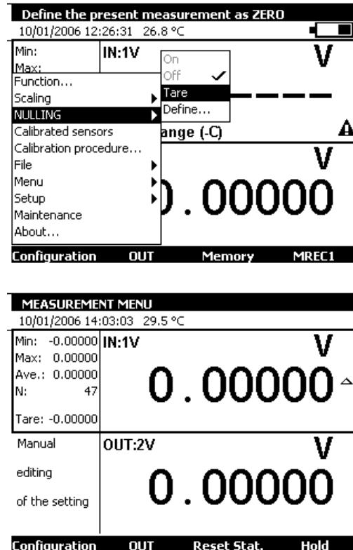
The **ZERO → Define...** menu is used to program the Tare value (positive or negative). This value is subtracted from the measurements:
