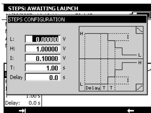
The parameters of a staircase are:
