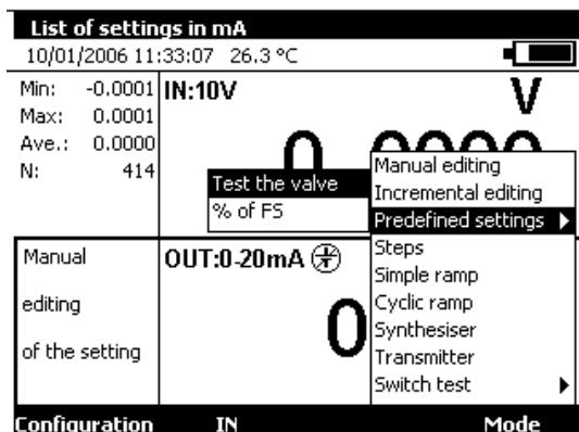
In the case of valve test, the predefined values are displayed in the left hand side of the transmission window. The icon is displayed in the right hand side of the window.
