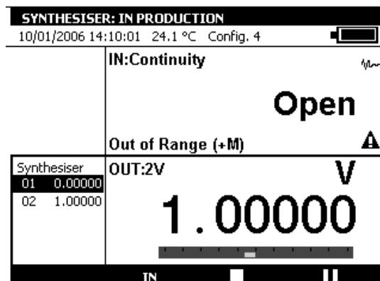
During generation, a progress bar indicates the state of progress. The function keys are used to control generation:
