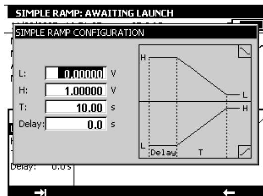
The parameters of a simple ramp are:
