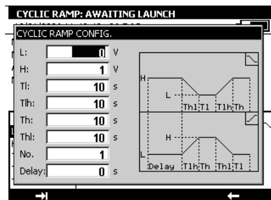
The parameters of a cyclic ramp are:
