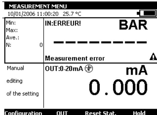
Connect the pressure sensor on the right-hand side of the unit (see chapter, side connectors). If this is not connected or is defective, an error message will be displayed.
