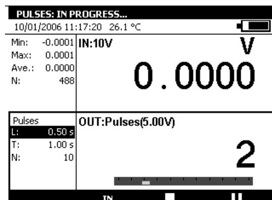
During pulse generation, a progress bar indicates the state of progress. The function keys can be used to control generation:
