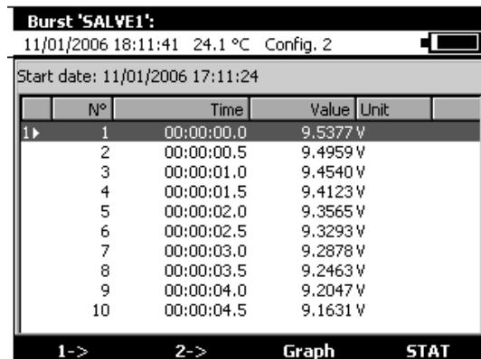
At this level, markers can be set (F1 and F2 function keys) and all values falling between these 2 markers can be displayed in graphical form.
