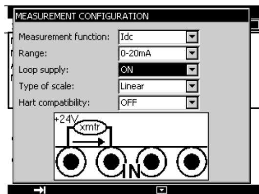
In this case, the CALYS 50 / 75 / 100 supplies a passive transmitter with 24 V and at the same time measures the current established by the transmitter.
