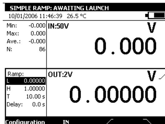
The key is used to launch an increasing ramp and the function key is used to launch a decreasing ramp. The default parameters of this mode are displayed in the left hand side of the transmission window. To change these parameters, press ENTER or use the **Configuration → Mode...** menus.
