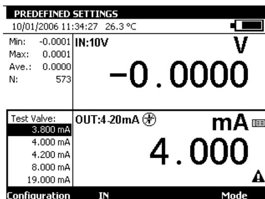
The Up/Down keys of the navigator can be used to select the setting from the list. The ENTER key transmits the selected setting. The Left/Right keys of the navigator are used to transmit the previous/next setting. The numerical keys 0 - 9 are used to enter the value to be transmitted on the keyboard.
