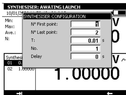
To edit the points to be synthesized, use the **Configuration → Synthesizer... → Points....** Menus.
