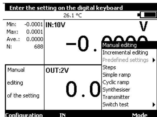
When the transmission window is open, the CALYS 50 / 75 / 100 is set by default to the **Manual edit** mode.
