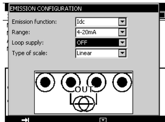
When the square law scale is selected, it must be activated by using the **Configuration → Set to scale** menus. Once "set to scale" is activated, the user enters the values to be simulated in a unit of the new scale.
