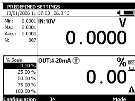
The icon indicates setting to scale. To display the scale applied, use the Configuration menu, then the "set to scale" menu.
