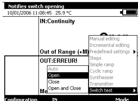
Once the type of detection is selected, every change of the selected type is detected and the measured value of pressure at the time of change is displayed.
