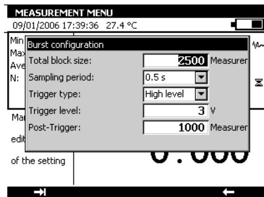
If high-level or low-level trigger is selected, the trigger level and number of data points to be stored after this trigger must be defined.
