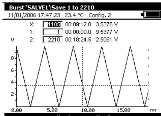
The left  $\triangleleft$  and right  $\triangleright$  arrow buttons can be pressed to move the cursor and read off the abscissa and ordinate values.
