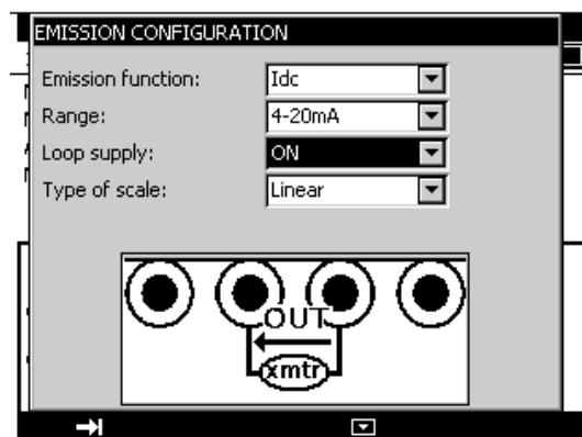
If the loop power supply is off, the CALYS 50 / 75 / 100 simulates a passive transmitter supplied with 24 V externally.
