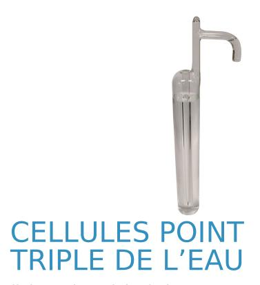
Cellules Point Triple de l'Eau, WTP cells
